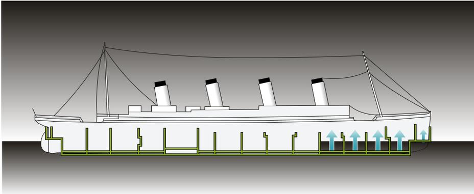
Damage caused by the collision with the iceberg affected five water-tight compartments (top).
